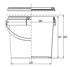
Measurements in millimetres
